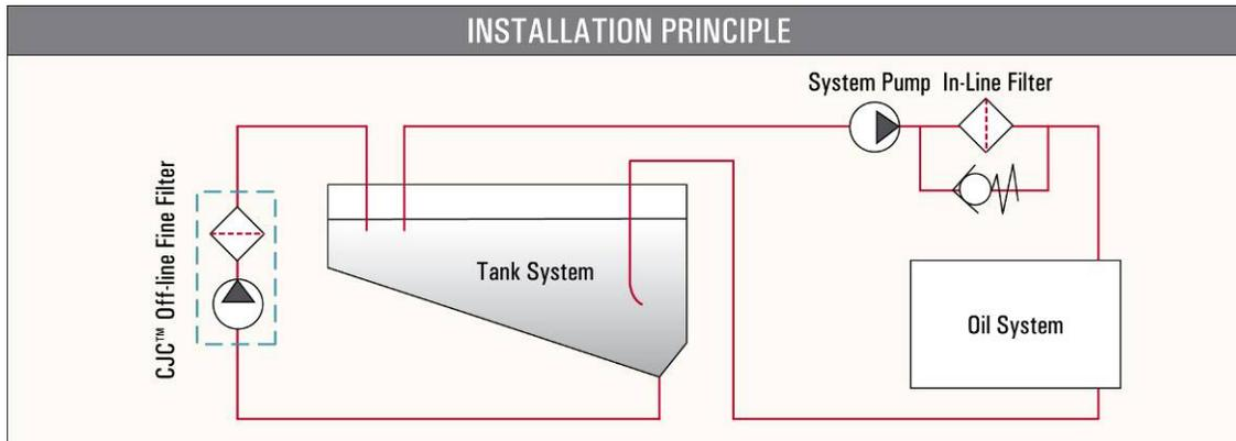
Schematic diagram of an offline oil filter installed on an oil system
