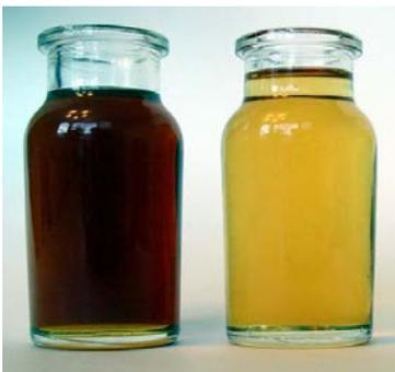
2) Degraded hydraulic oil compared to new oil (source: C.C.JENSEN)
